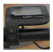
Please Note: Each pedal assist level has a pre-set maximum speed. When the set speed has been reached for the level of pedal assistance, the power to the hub motor will cease. Should you want assistance from the motor then you either need to reduce the pedalling activity and slow the bike, or press the + button to increase to a higher level of pedal assist.
